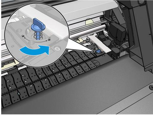
2. Remove both parts of the platen in the same way.
