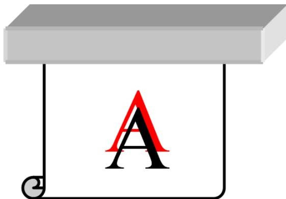
If the colors are misaligned in any direction, the printheads may be misaligned. This is likely if you have not aligned the printheads for a long time, or if there has been a substrate jam. Align the printheads if necessary
