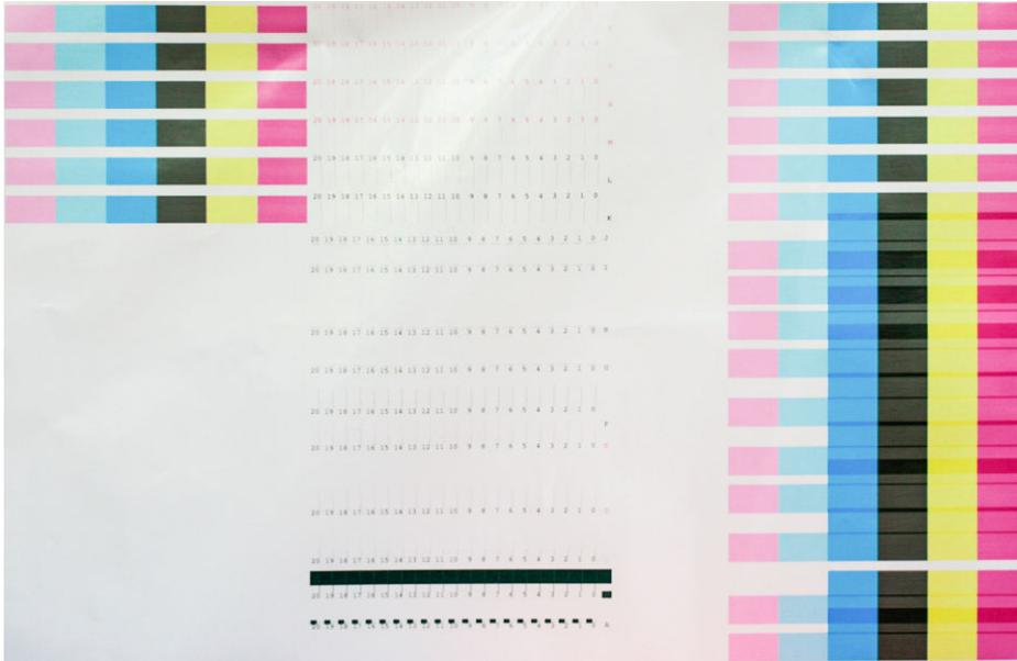
The printer prints 16 rows labelled from A to P. Inspect the print and write down the number of the straightest line in each row (for example, A:9).
