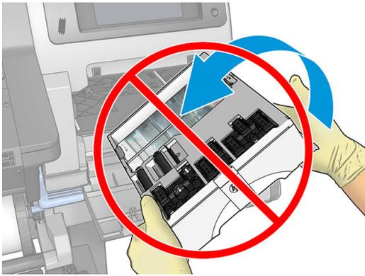
5. Remove the plastic cover from the new maintenance cartridge.
