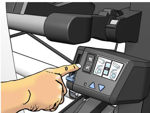
20. Press the **Enable** button on the front panel. The printer advances and calibrates the substrate.
