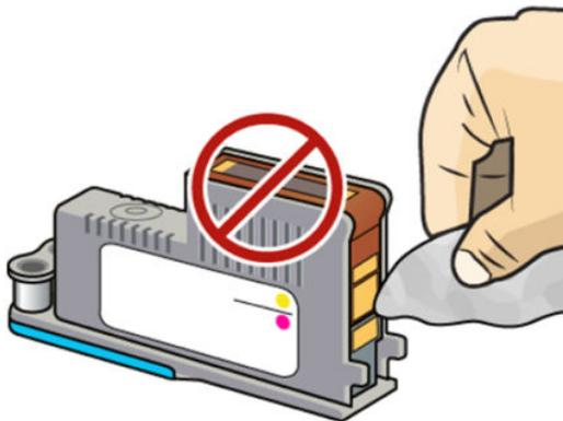
**⚠ CAUTION:** Do not touch the surface of the printhead that contains the nozzles, because the nozzles are easily damaged.
