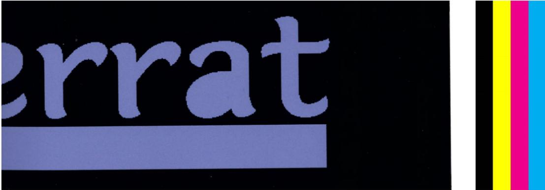
3. Add lateral color bars to the image, manually, before printing. In this case, you can either use the standard colors, or decide to include a particular color in which you have noticed the problem. The recommended width of each color bar is 5 mm.
