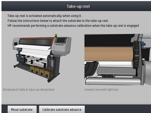
2. Load a core onto the take-up reel. Insert it first onto the right hub.
