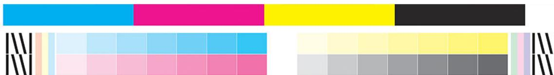
2. The test chart is scanned by the HP Embedded Spectrophotometer. If the scan cannot be completed successfully, a message is displayed on the front panel; see [Front-panel error codes on page 176](#).
