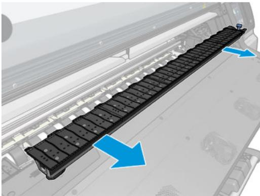
3. With care, smoothly place the two parts of the ink collector into the printer.
