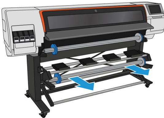
The spindle has a stop at each end to keep the roll in position. Remove the blue stop at the left end to mount a new roll (the stop at the other end of a 76 mm (3 in) diameter spindle can also be removed, if you wish). The stop slides along the spindle to hold rolls of different widths.
