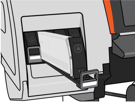
4. Lift the cartridge out of its drawer.
