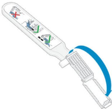
3. Load the sponge by positioning the sponge on the face of the carriage interconnect wiper with the shorter tab in the locating slot.
