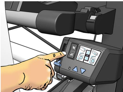
20. Tap the **Enable** button on the front panel. The printer advances and calibrates the substrate.
