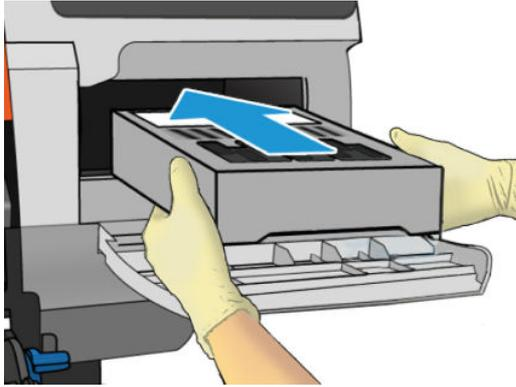
6. Push the maintenance cartridge in until it does not protrude from the slot. You will notice that the printer takes it; do not use excessive force.
