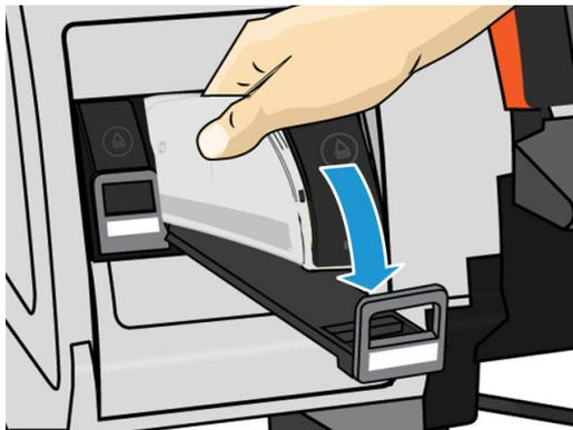
5. Slide the drawer and cartridge into the slot until they lock into position.
