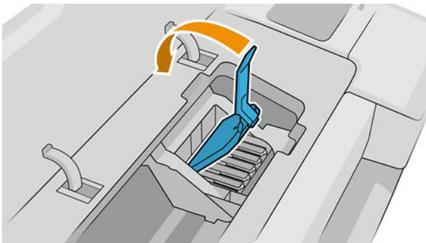
8. To remove a printhead, lift up the blue handle.
